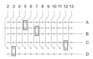
GOOD Setup. I/O Line Assignments to Channels: 3 to D, 5 to A, 7 to B, 12 to C
