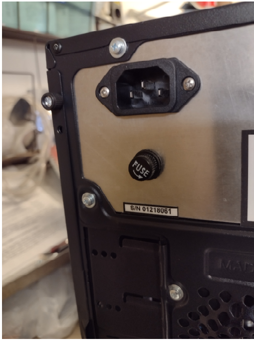
the fuse in place
