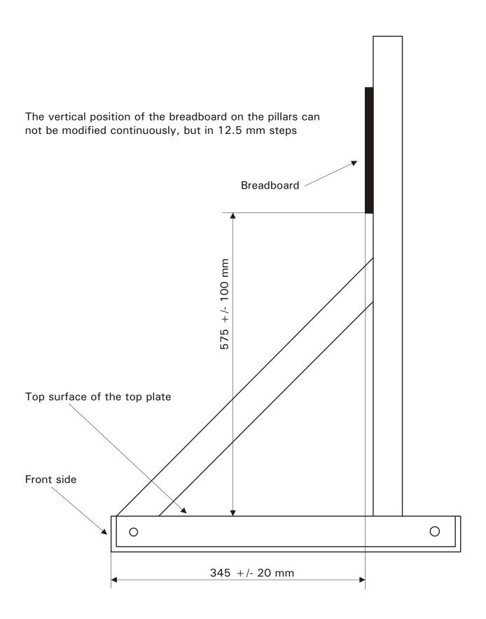
Size of the top plate by default: 1220 x 760 mm. To build a Vertical Spinning Disk Adaptor on a table, a specifically modified leg system is needed. It should be specified in the order.
