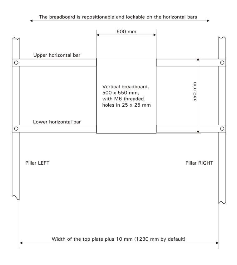
Size of the top plate by default: 1220 x 760 mm. To build a Vertical Spinning Disk Adaptor on a table, a specifically modified leg system is needed. It should be specified in the order.
