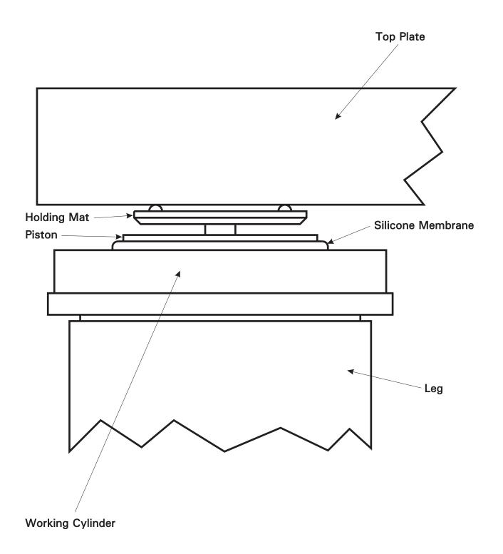
Figure 2. Parts of the Working Cylinder
