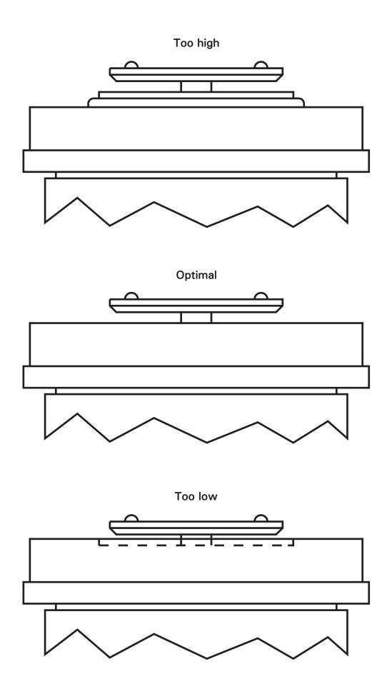
Figure 4. Adjusting the height of the Piston in the Working Cylinder
