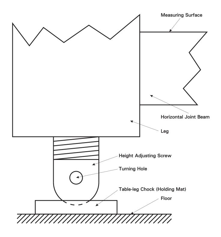
Figure 1. Horizontal level positioning of the leg system
