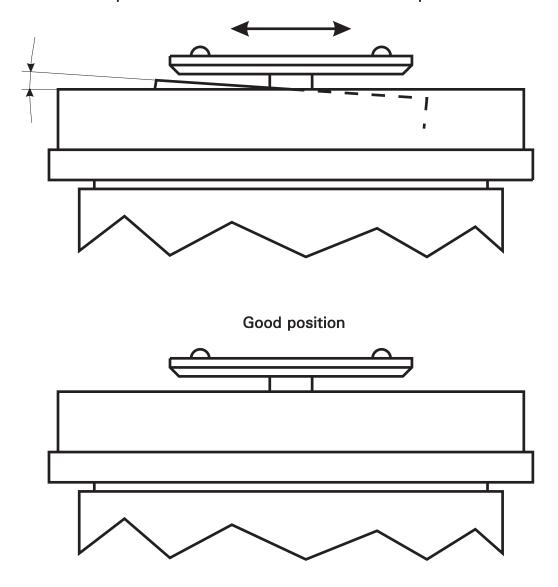
Figure 5. Vertical angle position of the Piston in the Working Cylinder
